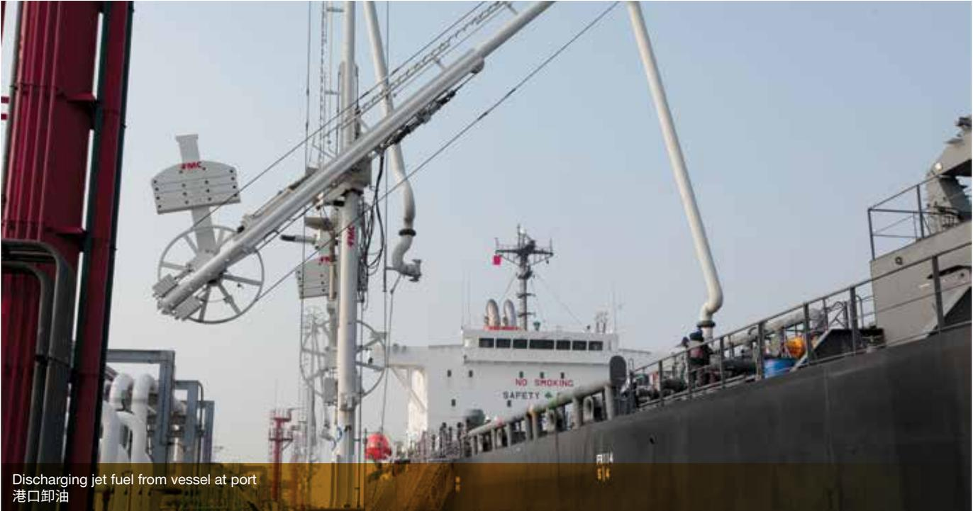
Discharging jet fuel from vessel at port
